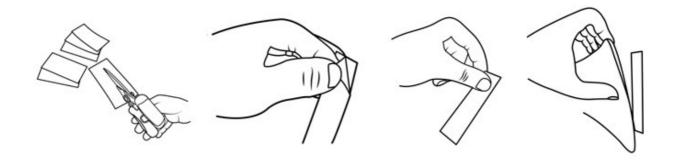
Cut the ULTRAMATE® tape to required size (cutting lengthways is one of the best options so you are left with two strips at 25mm wide) or use as-is, nip or round each corner, peel release paper and firmly press into place on the vehicle where the plates will attach paying particular attention to the edges. It does not matter what side you apply the to vehicle, however best results are by using the hook side to the vehicle and loop side for the number plates.
