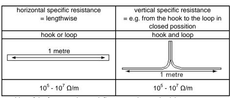
washing of the fasteners has no influence on the conductivity. tested in combination with clothing conform to EN 1149
